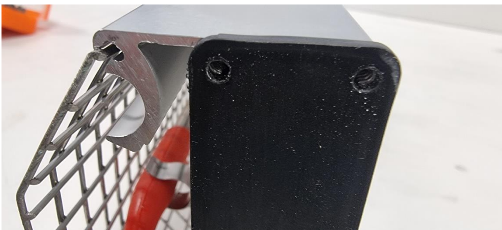
Photo 10 After IPX9. No water observed around sealing
