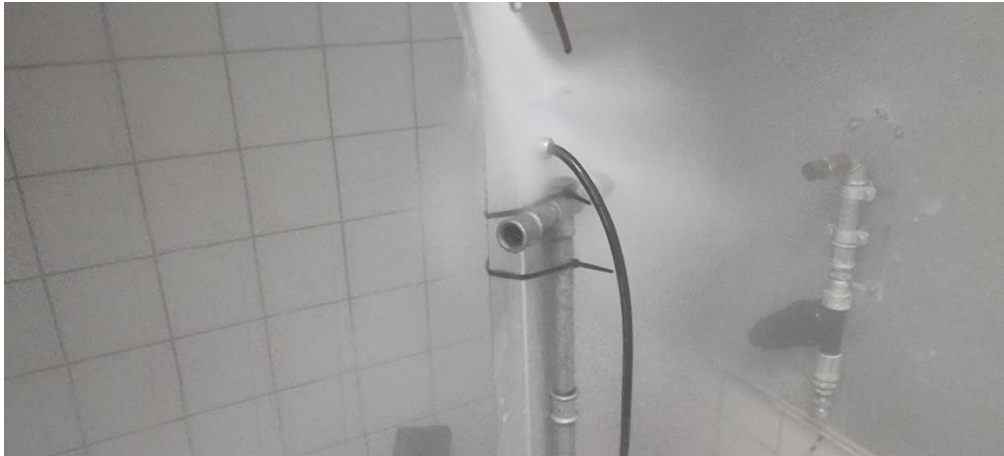
Photo 5 Enclosure protection, IPX9. Base cable inlet exposure.
