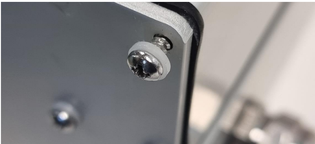
Photo 8 After IPX9. No water observed behind screw.
