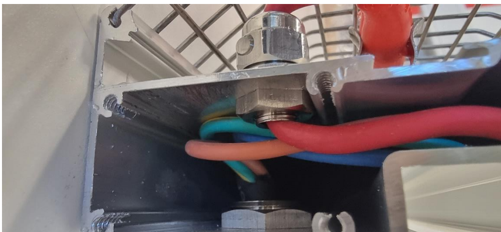
Photo 12 After IPX9. No water observed inside object
