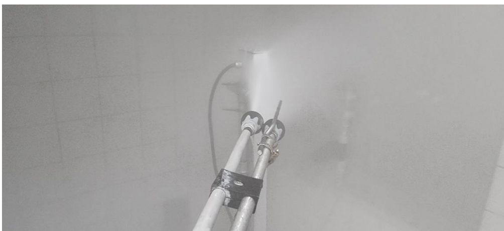
Photo 4 Enclosure protection, IPX9. top side exposure.
