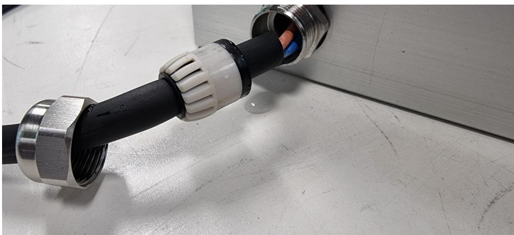
Photo 14 After IPX9. Water observed outside enclosure
