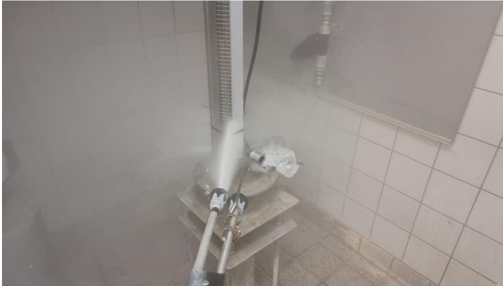
Photo 3 Enclosure protection, IPX9. Exposure.
